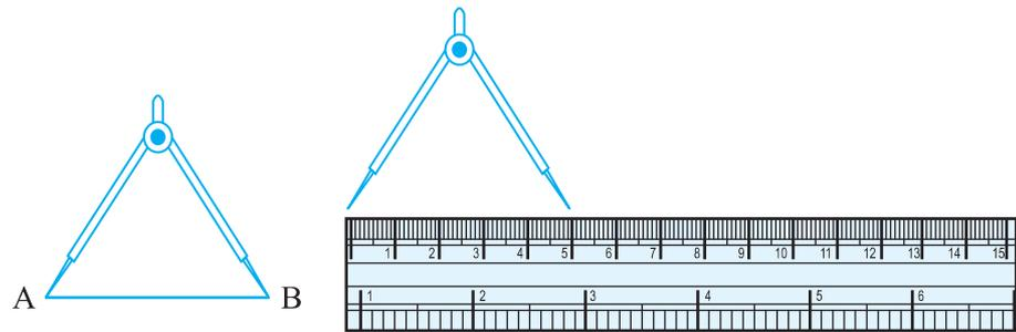
Open the divider. Place the end point of one of its arms at A and the end point of the second arm at B. Taking care that opening of the divider is not disturbed, lift the divider and place it on the ruler. Ensure that one end point is at the zero mark of the ruler. Now read the mark against the other end point.
